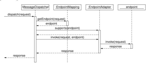
When a MessageDispatcher is set up for use and a request comes in for that specific dispatcher, said MessageDispatcher starts processing the request. The list below describes the complete process a request goes through when handled by a MessageDispatcher:
